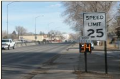
SPEED FEEDBACK SIGNS tell drivers their speed (measured by radar) and the speed limit on the road.
